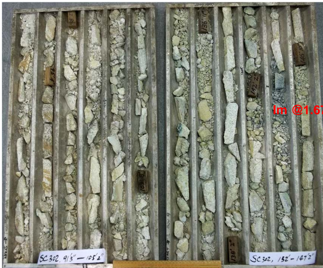
Photo photograph shows core slaps of SC302, 40.2-44.9m (132-147.2 feet), Cu @0.86% (sample OR11SC002). Core is currently stored in Victorian government core store.
